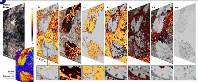
4K LIBS image of geological samples showing elemental distributions of Si, Fe, Cu, Al, Mg Ca and Ag (100 µs/point, resolution: 10µm)
