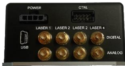
Modulation input SMB Connectors on the back of the laser head.
