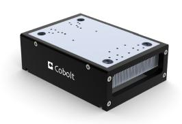
The value is the difference between the maximum operating laser base plate temperature (50°C) and the maximum ambient temperature at the air-heatsink interface (40°C), divided by the maximum power dissipated from the laser head (~20W). The mounting surface should be flat (within 0.05 mm over mounting surface).
