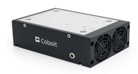
To ensure operation within given specifications, the laser head must be attached to a heatsink providing good thermal resistance. The value is the difference between the maximum operating laser baseplate temperature (50°C) and the maximum ambient temperature at the air-heatsink interface (40°C), divided by the maximum power dissipated from the laser head (~50W).
