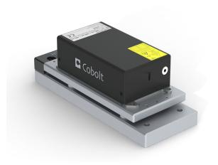
The TEC (thermo-electrically controlled) plate offers optimal temperature and wavelength stability for Cobolt lasers for applications which may be sensitive to air currents and vibrations from standard fanned (HS-o4) heatsink. The TEC plate is designed to accommodate all our Cobolt lasers. The TEC plate needs to be mounted on a suitable heatsink or
