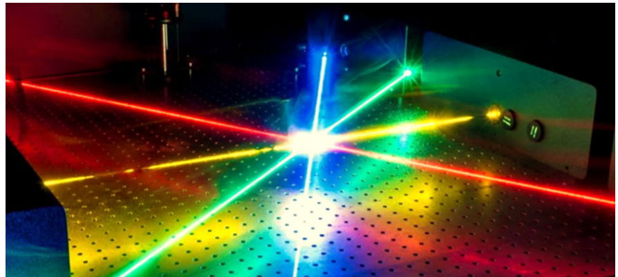
OPO technology provides laser light that is widely tunable across the visible spectral range. Figure courtesy of Jens Kiessling (Fraunhofer Institute for Physical Measurement Techniques).
