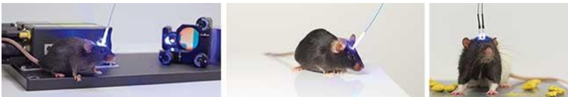
Cobolt MLD 473 nm used for excitation of opsins used in behavioral change studies of mice as they explore, and a rat experiencing reward. Courtesy of Cobolt.
