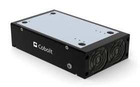
To ensure operation within given specifications the Laser Head must be attached to a heatsink providing good thermal resistance. This value is the difference between the maximum operating laser base plate temperature (50°C) and the maximum ambient temperature at the air-heatsink interface (40°C), divided by the maximum power dissipated from the laser head (~50W). The mounting surface should be flat
